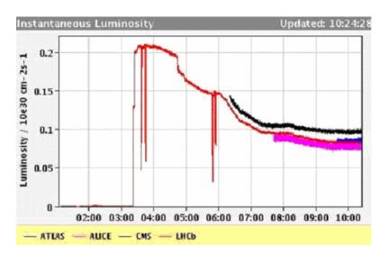
With such high bunch intensities the beam controllers must take extra care. If the beam becomes unstable the protons can go astray and plough into the sensitive particle detectors causing damage to the instruments. If instabilities grow the beams must be dumped quickly before all control is lost. This is why the gradual increase in luminosities has been a slow process.
