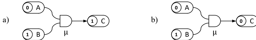
Fig. 3: The logic gate representing the AND operation:
