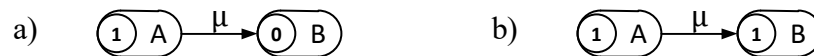
Fig. 1: a) Toma A is in state 1, toma B is in state 0. The function \mu is \theta[B_{\#}] := \theta[A_{\#}] . b) When \mu is selected for an update, this function is evaluated and the state of toma B changes to 1.
