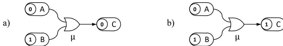
Fig. 4: The logic gate representing the OR operation:
